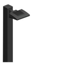
ALED Area Light mounts to 4" square steel poles at 15-20'. 1 to 4 ALEDs can be mounted to each pole. IESNA Full Cutoff, Fully shielded optics. 5 year warranty.
